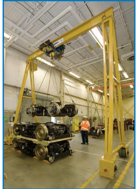
*Spanco Motorized PF-Series Gantry Crane*
