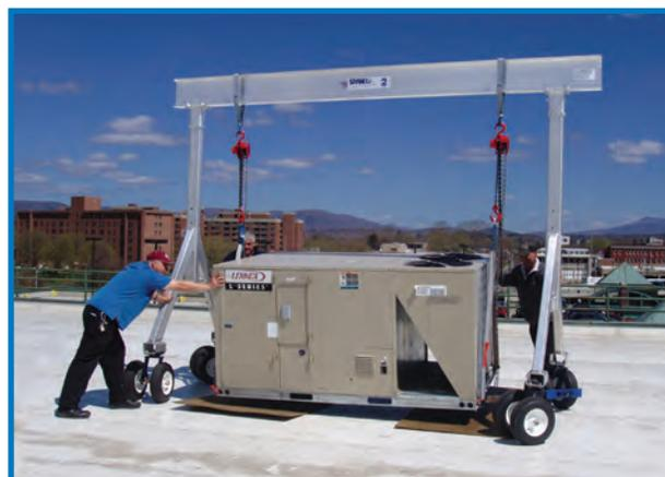
With systems as light as 116 pounds, just one worker can typically carry, assemble, and precisely position a Spanco Aluminum Gantry Crane almost anywhere — including rooftops. Designed to easily fit into or on top of most service trucks, these lightweight gantries carry up to 3 tons and are popular with contractors and in the HVAC industry.
