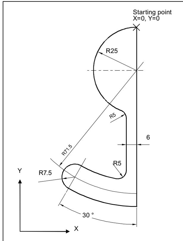
Figure 4-6 Workshop drawing of the contour, example 2
