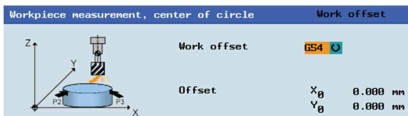
6. Press this vertical softkey to save the tool position P1 in the coordinate system.
