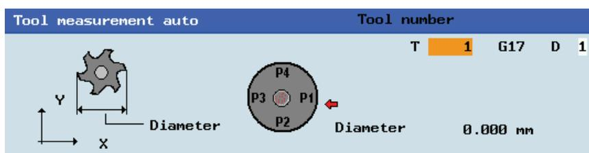
10. Manually position the tool in the vicinity of the probe in a way that the collision can be avoided when the probe is traversing.
