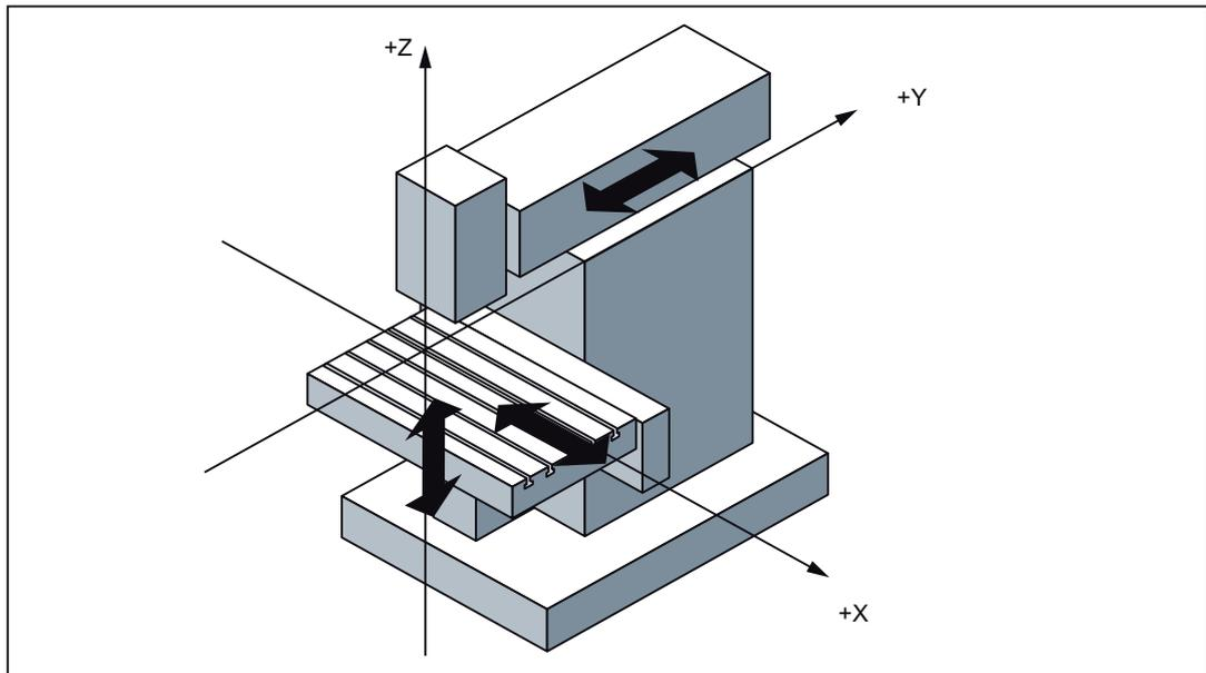
The origin of this coordinate system is the **machine zero**. This point is only a reference point which is defined by the machine manufacturer. It does not have to be approachable.
