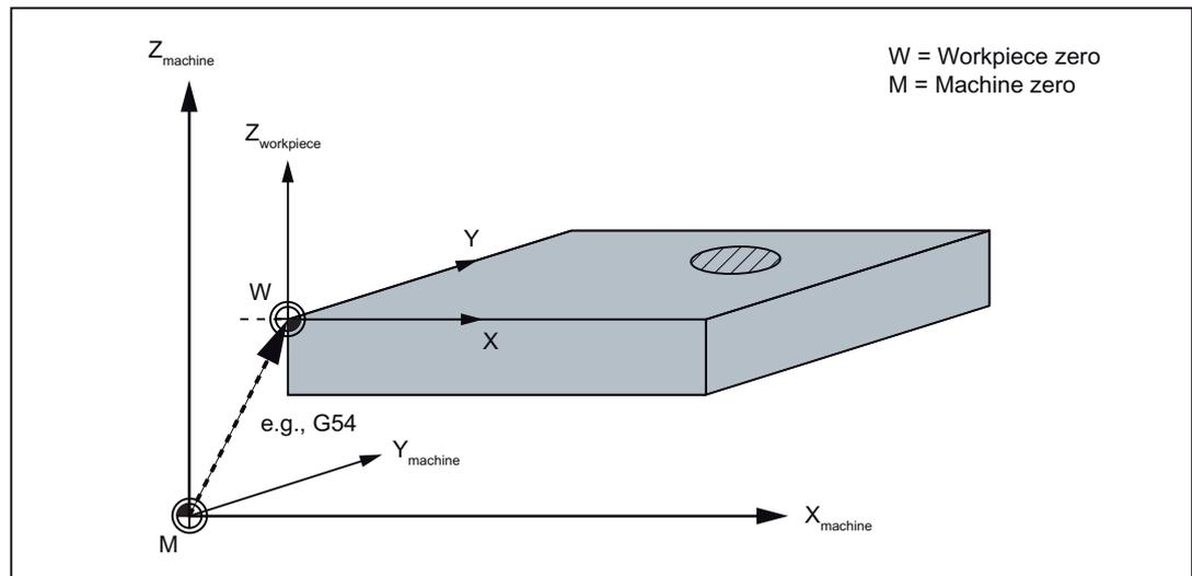
**Current workpiece coordinate system**
