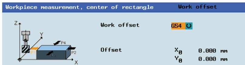
6. Press this vertical softkey to save the tool position P1 in the coordinate system.
