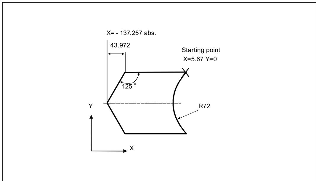
Figure 4-5 Workshop drawing of the contour, example 1
