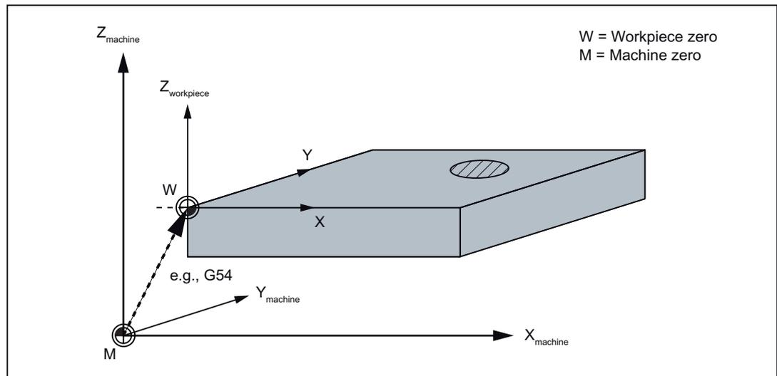
**Current workpiece coordinate system**
