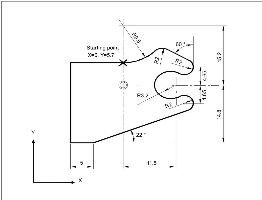
Figure 4-7 Workshop drawing of the contour, example 3
