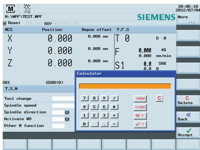
For calculating, the four basic arithmetic operations are available, as well as the functions "sine", "cosine", "squaring" and "square root". A bracket function is provided to calculate nested terms. The bracket depth is unlimited.
