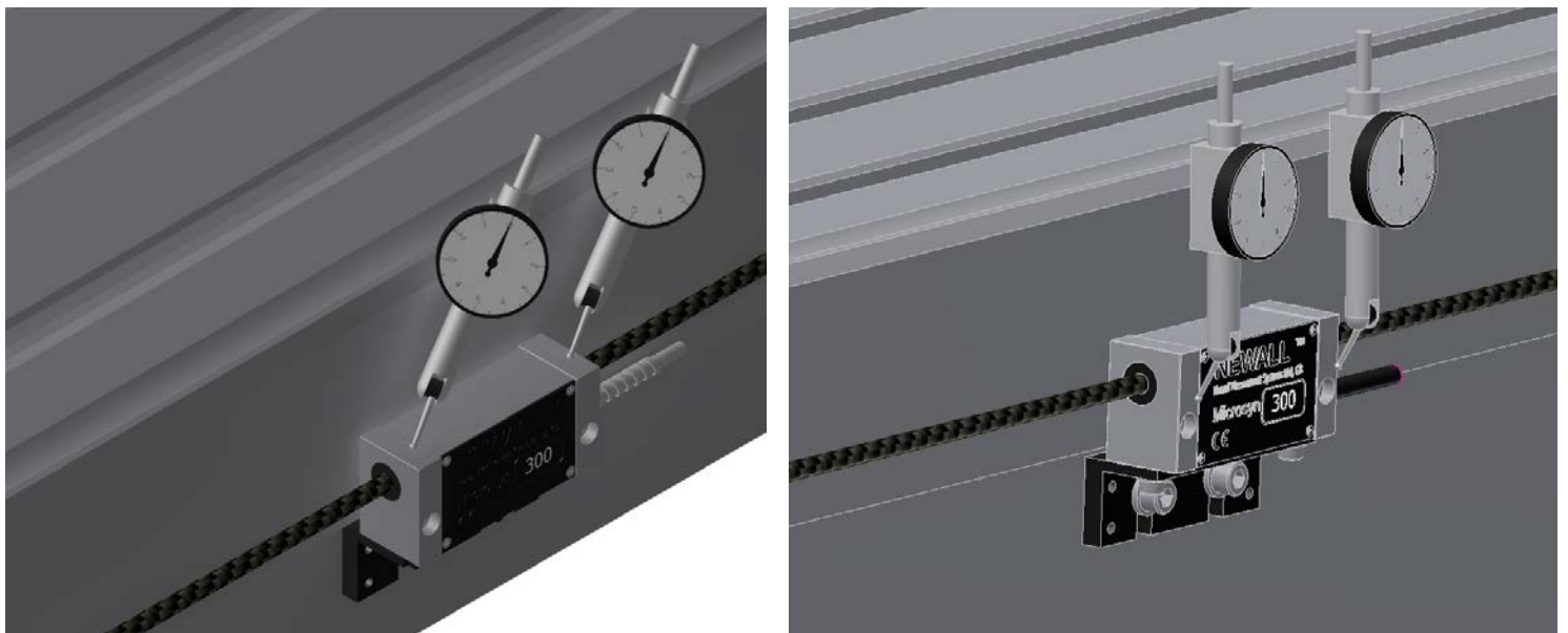
Figure 4.2 - Alignment of the Microsyn 300 Reader Head
