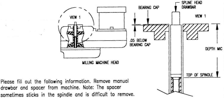
A. With the quill all the way retracted and lock (home position on CNC) depth mic from the top of the bearing cap to the top of the spindle. What is this distance minus .05?
