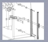
This option provides the machine operator positional feedback on the control when the knee is manual moved.
