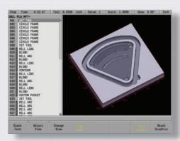
Bring a brainstorming session to life with simple features that reduce programming time. DXF file input allows the operator to import part geometry directly from a CAD file. After the DXF file has been loaded, save on MILL**PWR<sup>G2</sup>'s** large internal memory, USB or on your PC (via Ethernet) for easy retrieval later on.
