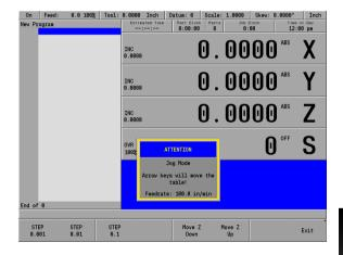
▶ Press the appropriate ARROW key (or soft key) to move the table in the direction required for the axis move. The table will move at the currently active jogging speed. The table will move until the ARROW key is released.
