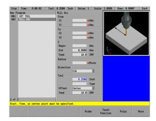
Once a step has been programed in the program dialogue and the USE key has been pressed, if the data in any field has been entered incorrectly, that field will display a yellow warning symbol.
