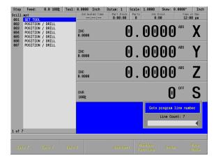
MILLPWR $^{G2}$  will automatically pause at points that require action to be taken (e.g., change tools). After each task has been completed, press the  ${\bf 60}$  key.
