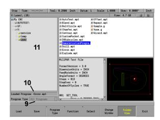
The MILLPWR<sup>G2</sup> can save programs to a USB device, or to network drive (e. g. a PC) as well as to the MILLPWR<sup>G2</sup> User folder.
