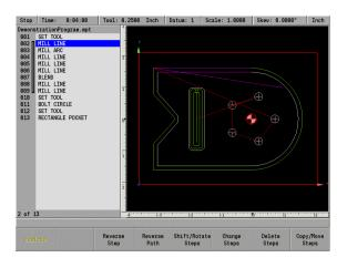
Machining a part in PGM mode will show the soft keys to easily select between 2D Line, 3D Line and 3D Solid without having to open the View Setup dialogue.
